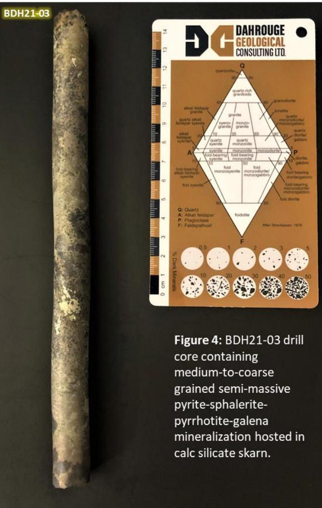
**Figure 4:** BDH21-03 drill core containing medium-to-coarse grained semi-massive pyrite-sphalerite-pyrrhotite-galena mineralization hosted in calc silicate skarn.
