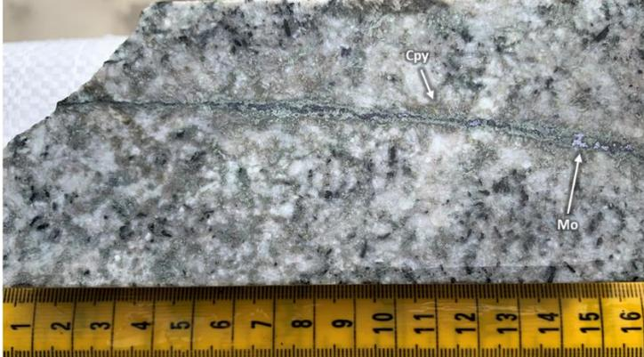
**Figure 1:** Photographs of HQ-sized core intervals from LAV22-006 showing Cu-Skarn and Cu-Mo porphyry style mineralization.
