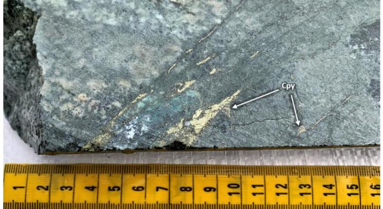
LAV22-006 – Magnetite(Mt)-Chalcopyrite(Cpy)-Pyrrhotite(Po) Skarn at 167.10m
