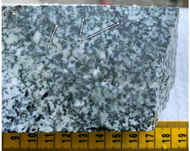
LAV22-006 – Molybdenite(Mo)-Chalcopyrite(Cpy)-Chlorite(Chl)-Sericite(Ser) Vein at 177.17m
