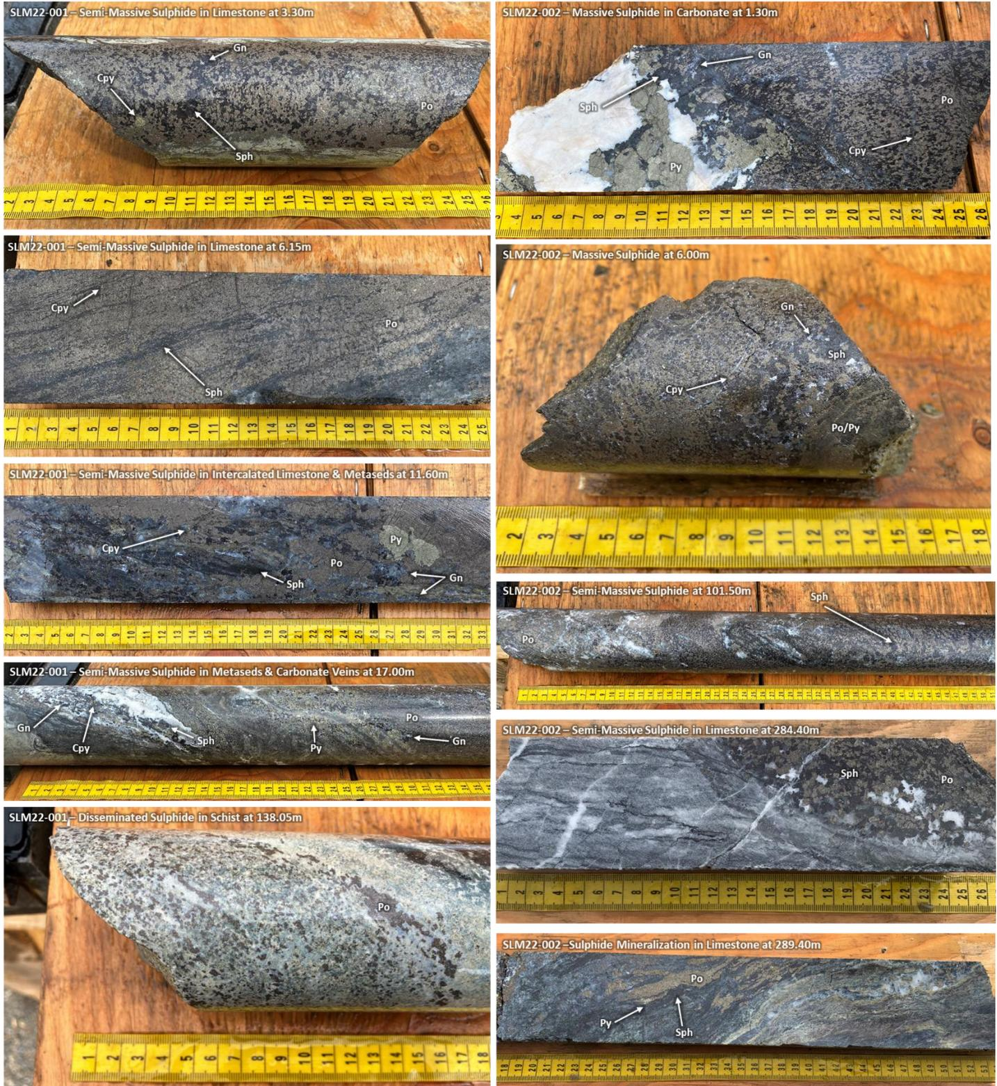
**Figure 1:** Photographs of representative 2022 HQ-sized core intervals from SLM22-001 and SLM22-002 of base metal sulphide (Chalcopyrite = Cpy; Galena = Gn; Sphalerite = Sph; Pyrrhotite = Po; Pyrite = Py) occurrences at the Jackie Target, Silver Lime Project.
