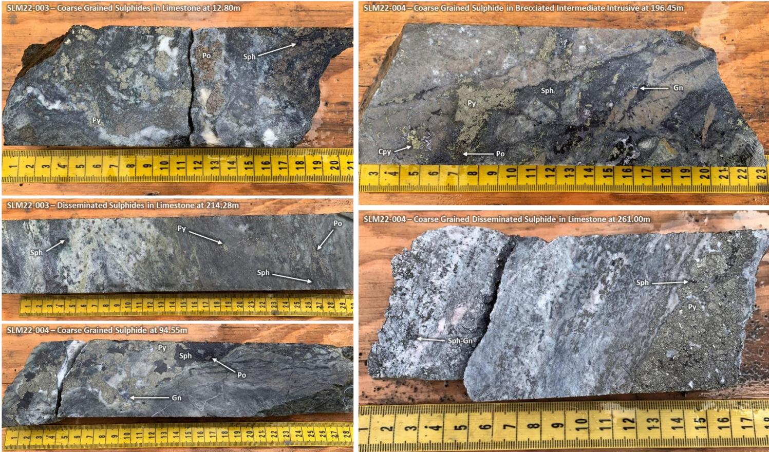
**Figure 2:** Photographs of representative 2022 HQ-sized core intervals from SLM22-003 and SLM22-004 of base metal sulphide (Chalcopyrite = Cpy; Galena = Gn; Sphalerite = Sph; Pyrrhotite = Po; Pyrite = Py) occurrences at the Jackie Target, Silver Lime Project.
