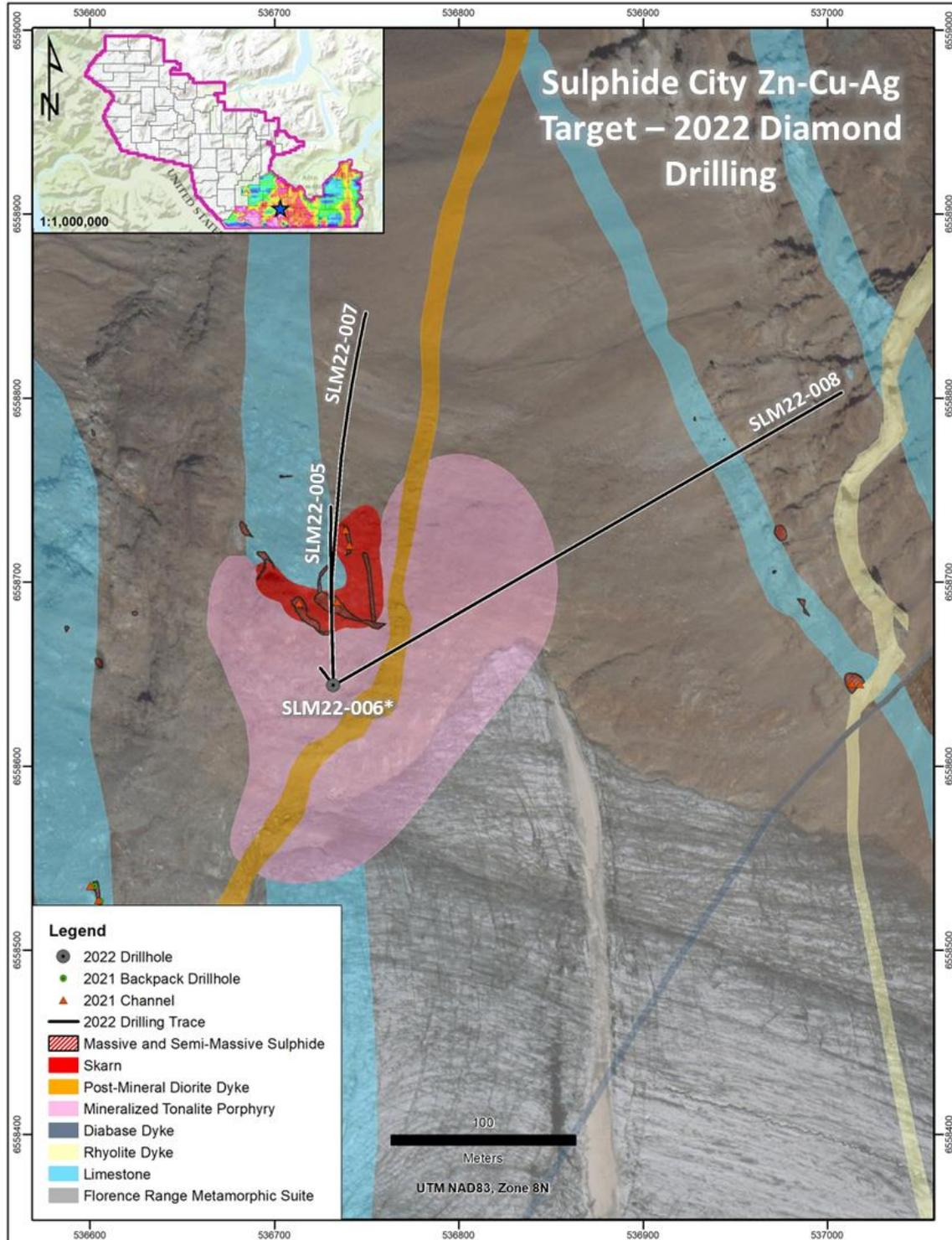
**Figure 2:** Planview geological map of the Sulphide City Target at the Silver Lime Porphyry-CRD Project showing 2022 diamond drilling progress, surficial extents of the syn-mineral tonalite porphyry and post-mineral diorite dyke and mapped massive to semi-massive sulphide occurrences. \* indicates a vertical drill hole and hole SLM22-005 was lost at 137 metres depth (EOH).
