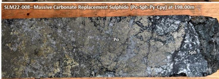
**Figure 1:** Photographs of 2022 HQ-sized core intervals from the Sulphide City Target showing representative tonalite porphyry, porphyry mineralization/alteration, and base metal sulphide skarn and carbonate replacement mineralization. (Chalcopyrite = Cpy; Molybdenite = Mo; Galena = Gn; Sphalerite = Sph; Pyrrhotite = Po; Pyrite = Py; Potassic Alteration= K+; Biotite=Bio; Quartz-Sericite-Pyrite Alteration = QSP; Massive = MS; Carbonate Replacement Mineralization = CRM).
