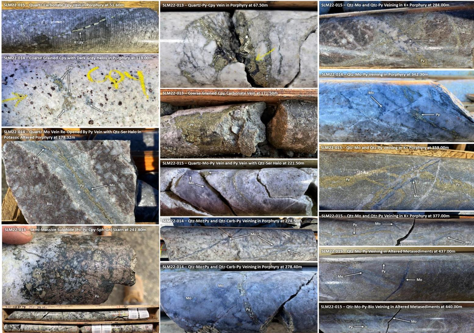
**Figure 1:** Photographs of 2022 HQ-sized core intervals from the Sulphide City Target showing representative sulphide porphyry, skarn, and porphyry-type vein-hosted mineralization. (Chalcopyrite = Cpy; Molybdenite = Mo; Galena = Gn; Sphalerite = Sph; Pyrrhotite = Po; Pyrite = Py; Sericite = Ser; Potassic Alteration = K+; Biotite=Bio; Quartz-Sericite-Pyrite Alteration = QSP; Semi-Massive = SMS; Massive = MS; Quartz = Qtz; Carbonate = Carb).
