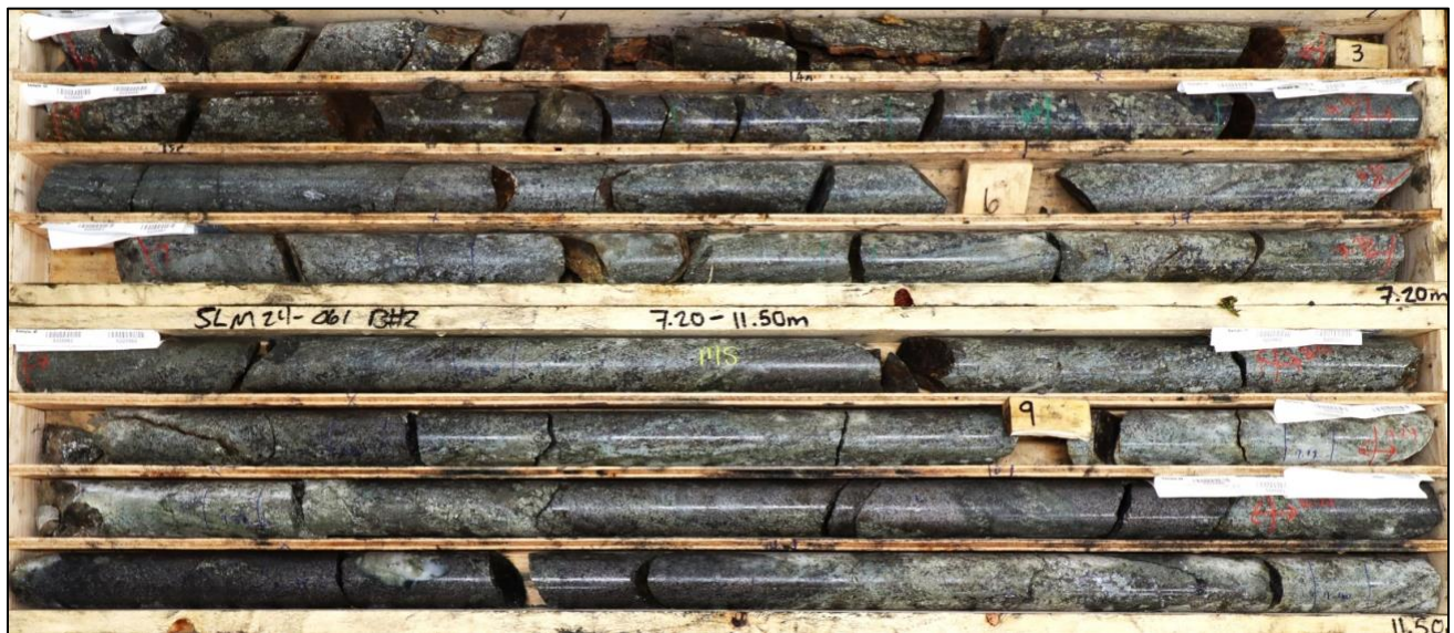
Figure 1: A photograph of the continuous 11.8-metre interval of massive sulphide (sphalerite-pyrrhotite-pyrite+/-chalcopyrite-galena-rich) skarn mineralization in Sulphide City-Whaleback hole SLM24-061.
