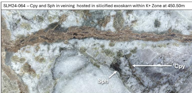
Figure 2a: Photomicrographs of prospective porphyry-skarn mineralization and alteration textures observed in drill core collected from the Sulphide City Porphyry Target in 2024.
